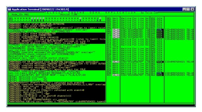
In the above example the top right shows single character channel status for each channel on each E1 trunk. Down the right hand side is a more detailed channel status and additional channel/call specific information. The main area rectangular area on the bottom left is the scrolling log window, showing all calls to the applog(), errlog(), tracelog() and similar functions to display scrolling messages.
